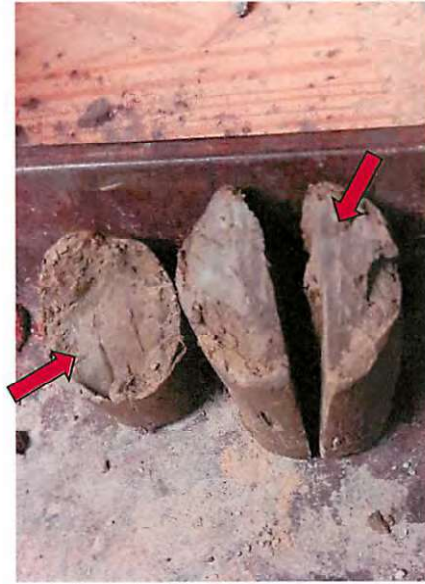
Slickenside (shiny shear surface) B-3, SS-8
